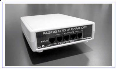
The PGE can utilise up to 5 analogue ports and 1 STRB / Reals board to facilitate the simultaneous paging of 99 ports. 1 analogue port is included in the (trigger) group, with 19 other digital extensions. This analogue port is connected via the STRB / Reals relay to the input of the Paging Group Expander and provides power to operate the Paging Group Expander, as well as the audio input to the other ports on the device (see diagram below).
