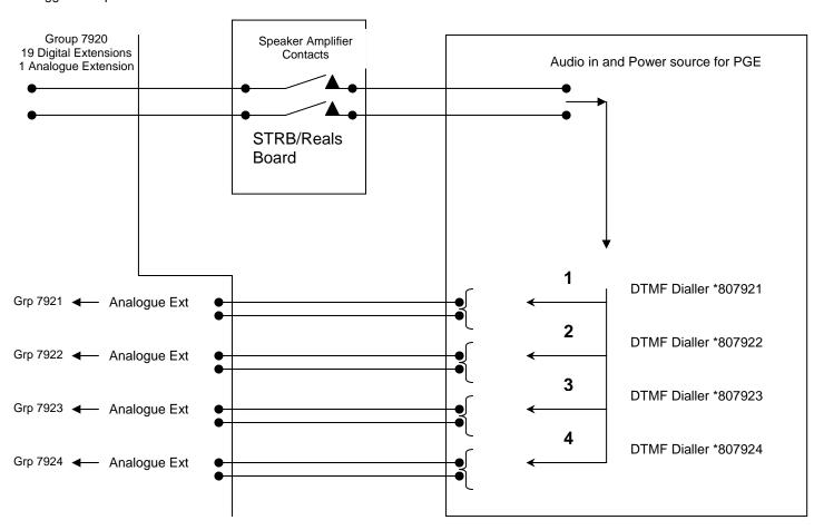
Note: With internal links LK1, LK2, LK3 & LK4 NOT fitted, the PGE dials group pilot numbers \*807921,\*807922, \*807923 and \*807924. With the links fitted it dials group pilot numbers \*80861, \*80862, \*80863 and \*80864.
